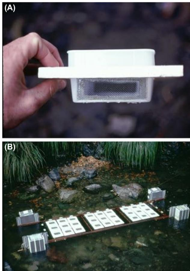
**FIGURE 18.2** Grazer enclosures used to manipulate densities of small benthic grazers. (A) Each enclosure is  $\sim 500 \text{ cm}^3$  with sides screened with 1-mm<sup>2</sup> mesh and fitted with a styrofoam collar for flotation. (B) Floating rack holding 27 enclosures tethered in a stream run of Big Sulfur Creek, California, USA. Photos: Gary Lamberti (see also Lamberti *et al.*, 1987b).
