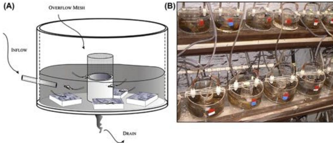
**FIGURE 18.5** Small flow-through streams for predation experiments. (A) Drawing (by Peter Ode) and (B) photograph of two different designs of circular chambers for *Advanced Method 1* that could be used in the laboratory or streamside to contain small animals. (B) Photo: Joanne Peckarsky.
